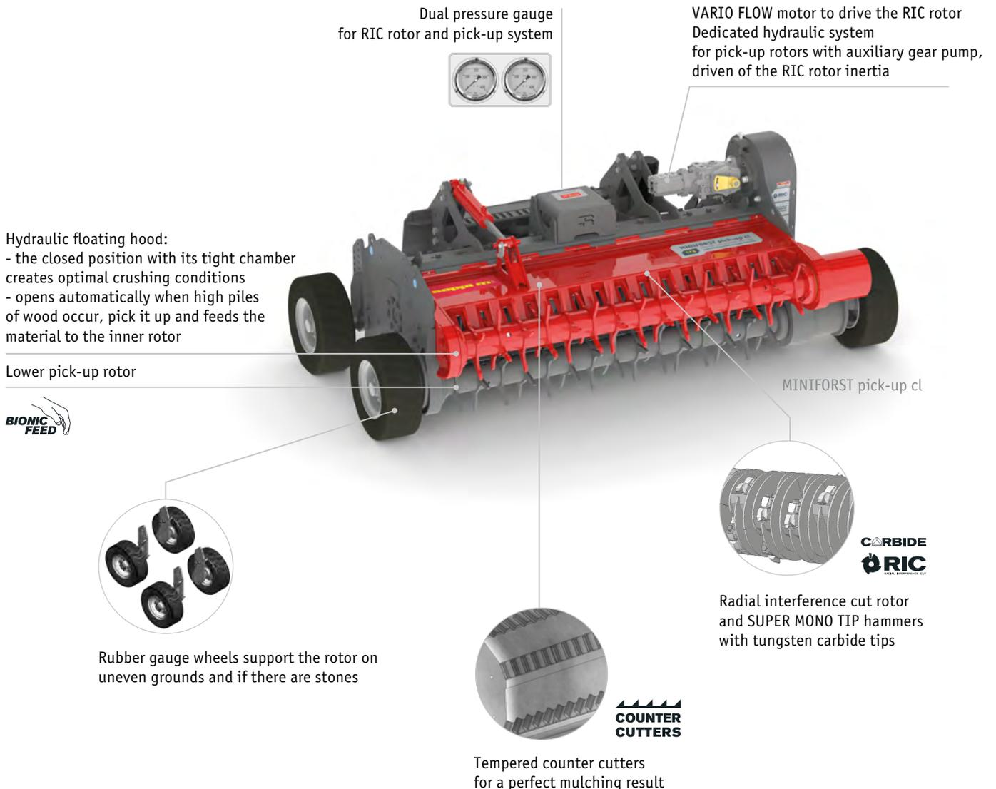
Safety Note: MINIFORST pick-up cl may be raised to a maximum of 50 cm [20 inch] and should be only used with stone impact protected cabins.
